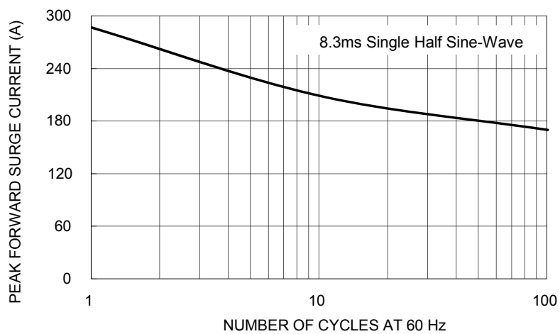
FIG. 3 MAXIMUM NON-REPETITIVE FORWARD SURGE CURRENT
